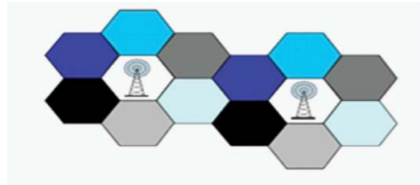
Exhibit 145: Base Stations Communicate with Each Cell on a Different Frequency (Represented by Different Colors), to Stop Interference.
